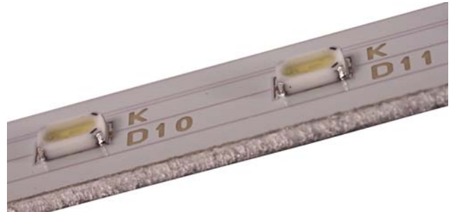
Figure 1. Closeup of LED Backlight Assembly
